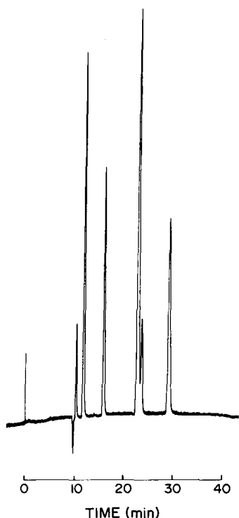
Fig. 1. Chromatogram illustrating refractive index artifact occurring in absorbance detection upon injection of standard test mixture dissolved in methanol into a methanol-water (75:25, v/v) mobile phase. Characteristic derivative-shaped response from absorbance anomaly is seen at a retention time of 10 min.
